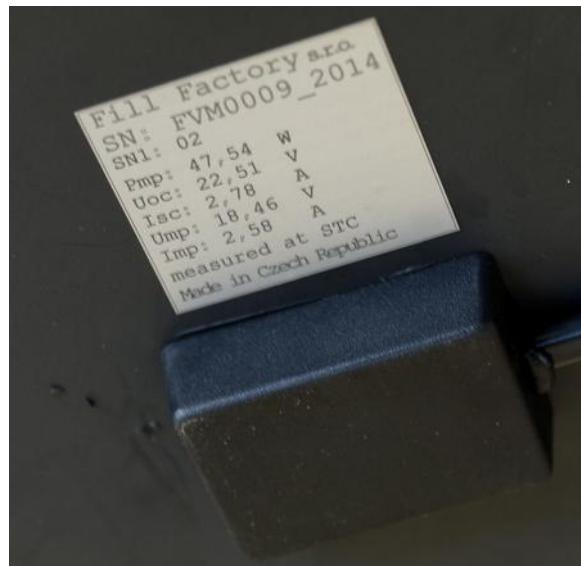
Marking of backsheets in PV laminate (e.g. our [irradiation sensors](#))
